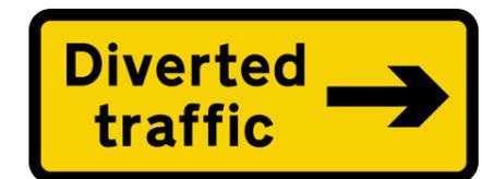
Sign used in advance of a junction to indicate the direction diverted traffic should take at the junction ahead (Ref: 2703)
