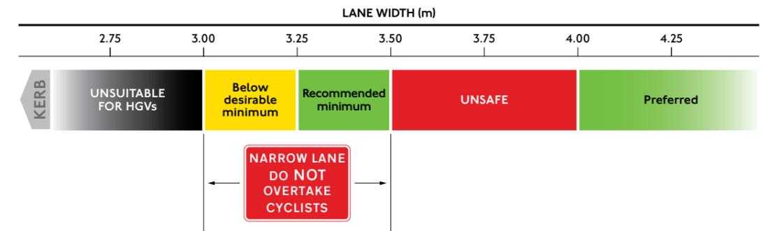
Widths between 3.25 metres and 3.5 metres will allow buses and HGVs to use the lane but it will not be possible for them to overtake cycles.
